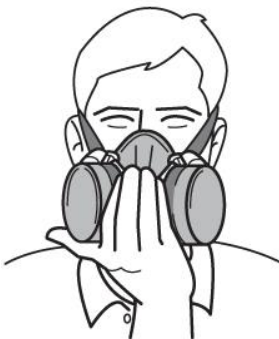
Positive pressure fit check
