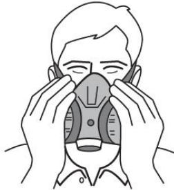
Negative pressure fit check
